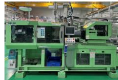
Injection molding machine using low pressure molding technology
