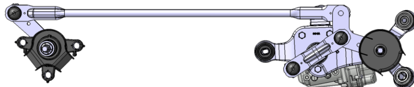
brushless motors for wiper control systems
