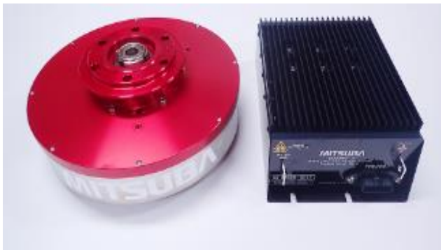
Solar car drive system Adopting amorphous materials and flat wires - Optimized for 98% maximum efficiency
