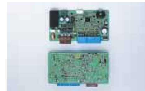
Power sliding door controller containing lead-free solder
